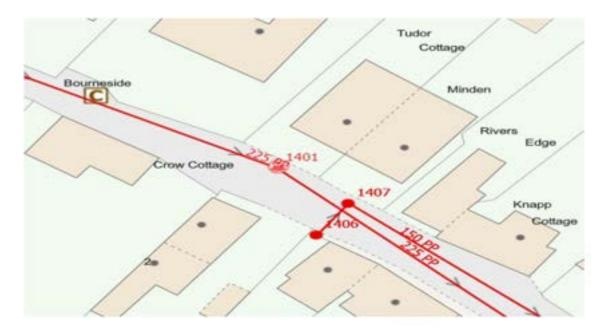
8. Extend the rising main from the micro pumping station in manhole 0503 to join the 150mm rider sewer at manhole 1407 – work to be completed Autumn 2024, dependant on power supply.
