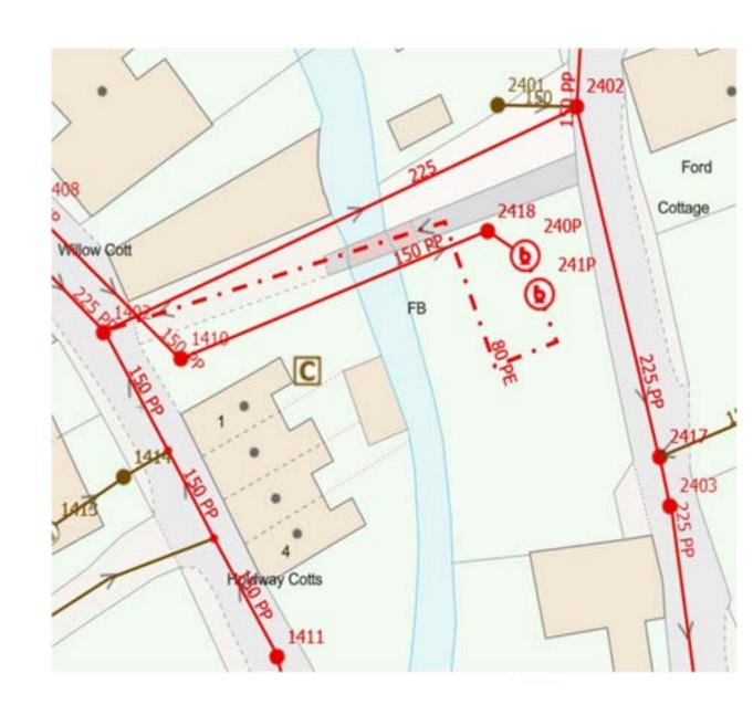
11. Install two long radius bends at manhole 1402 and one long radius bend at manhole 2402 to improve conveyance of flows – work to be completed September 2024
