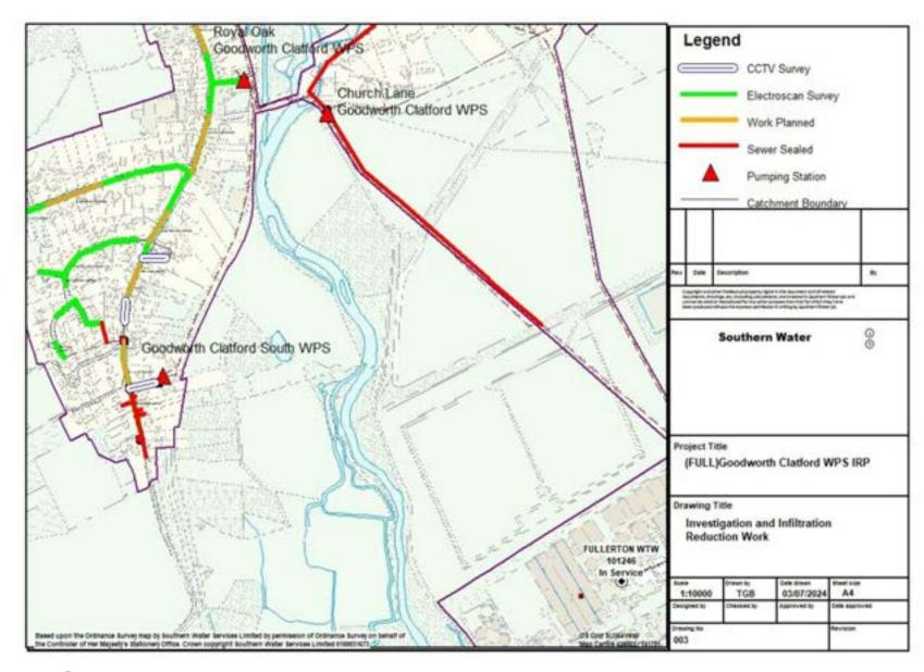
Note – sewers shown as surveyed by cctv or electroscan with no corresponding sealing work have been determined to not require rehabilitation.
