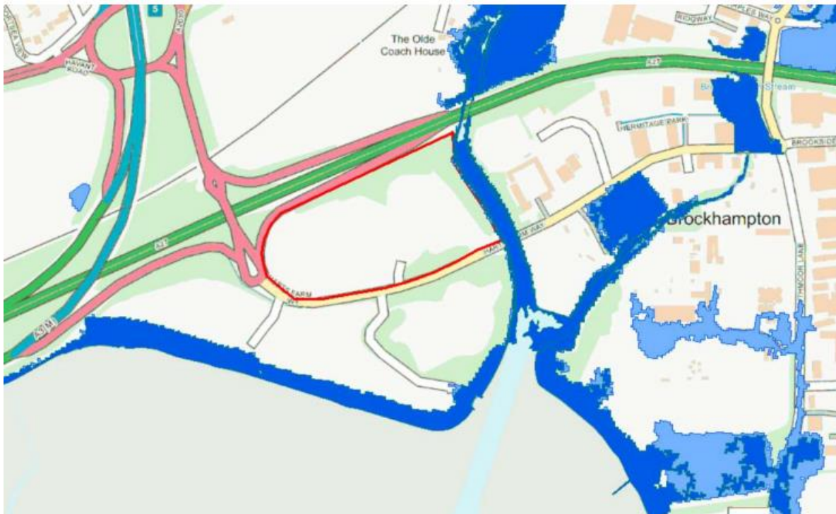
Figure 2-31 - Flood Map for WRP Site showing Flood Zone 2 (light blue) and 3 (dark blue)
