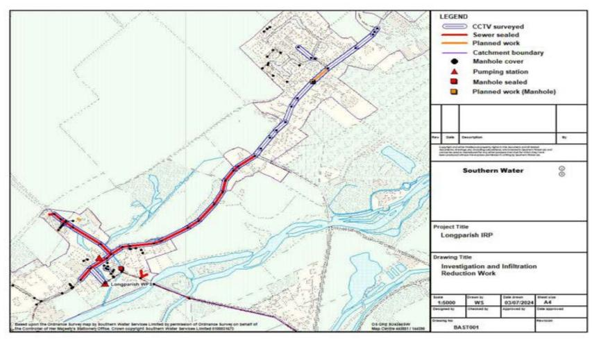
Note – sewers shown as surveyed by CCTV or electroscan with no corresponding sealing work have been determined to not require rehabilitation.
