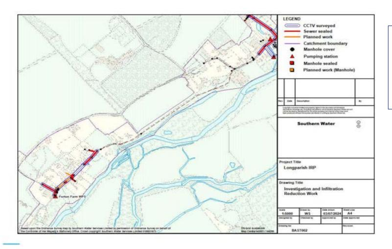
Note – sewers shown as surveyed by CCTV or electroscan with no corresponding sealing work have been determined to not require rehabilitation.
