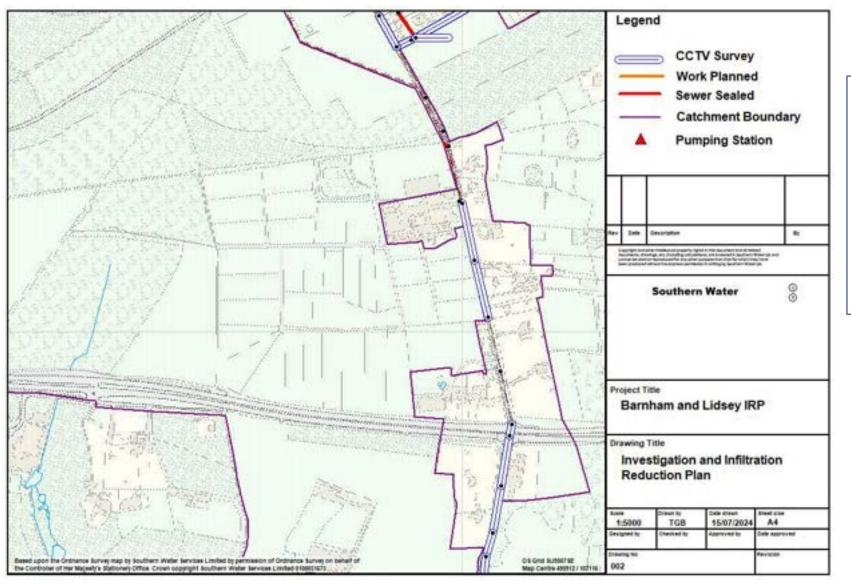
Note – sewers shown as surveyed by cctv or with no corresponding sealing work have been determined to not require rehabilitation. The use of storm harvester data will be used at some point in the future to target inspections and find infiltration
