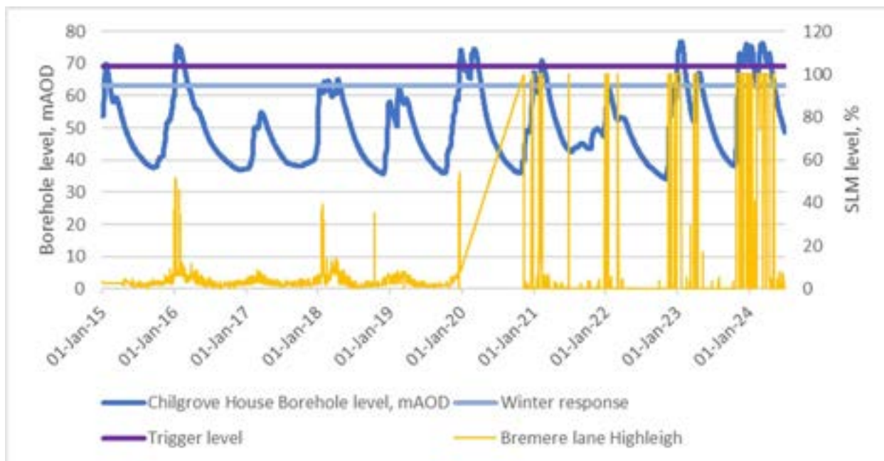
Figure 4.1 - Groundwater levels from 2015 to 2024
